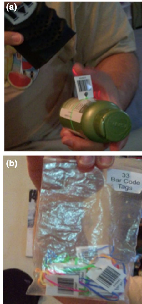
Fig. 4 How a barcode reader was used to recognize the barcode tag on the bottle (left). Reusable barcode tags (right)
